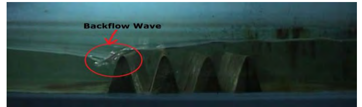
Fig. 3 Contrarily backflow wave ( w/h = 0.5 · D/h = 0.75 )
